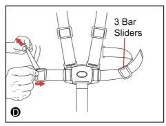
(16) To tighten or loosen the shoulder straps, slide the 3 bar sliders up or down to adjust to the desired fit. Always adjust the harness strap when changing the seating positions of the child (Fig E).
