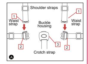
(13) Push both buckle tongues (1+2) into the buckle housing (3) until the buckle tongues lock into position (Fig B).
