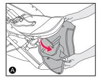
(10) The Foot Barrier is under the Footrest, take it out as shown in Fig. A.Put the bumper bar go through the Foot Barrier, then attach the bumper bar to stroller frame, as shown in Fig B.Attached the Foot barrier to the side of the seat with the two Snaps at each side, as
