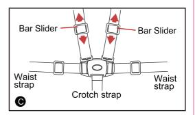
(15) To tighten or loosen the waist straps, hold and lift the 4 bar sliders, then pull the harness strap to adjust to the desired fit. The waist strap needs to fit firmly around the child (Fig D).
